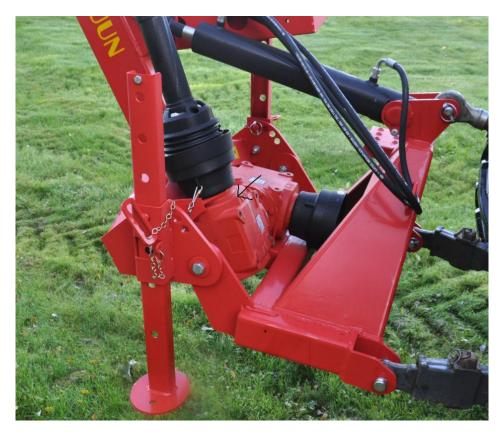
2. Release four screws securing the safety funnel and the mounting bracket to the double gearbox pointing away from the tractor. Release the long screw which secures the bracket to the pump mount. Remove the safety funnel and the old bracket. Take care of the safety funnel and two washers for screws that secure the safety funnel.
