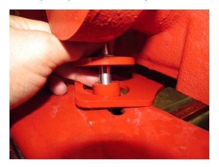
4. Screw the bracket to the gearbox as shown in the picture.
