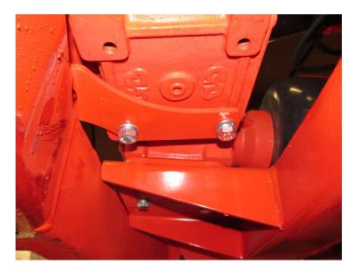
5. Center the screw with the spacer washers on the picture two and screw in place with a nut on the underside of the pump attachment. This screw can now be properly attached without the gearbox being locked.
