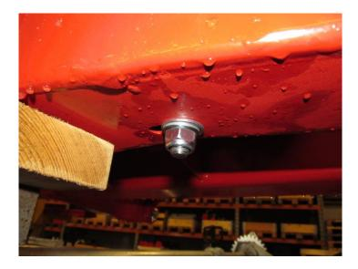
6. Put the safety funnel back and fasten it with two new screws that are shorter than four screws before. Use washers which were picked off when the safety funnel was dismantled.
